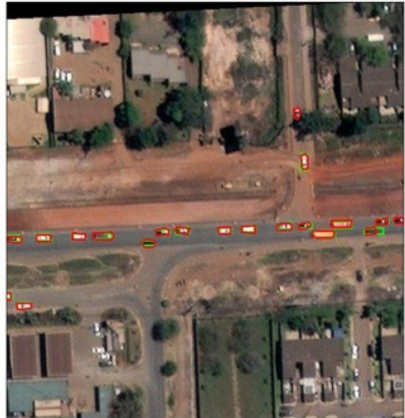
Satellite image of a street in Kenya illustrating vehicle identification process © Maxar
